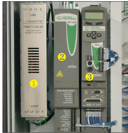
The remote electronics for a GSX actuator require very little space. For IMM mold applications, they’re often put in a small rolling cabinet that sits next to the machine. 1. Line filter, 2. Power supply, 3. Servo controller into which you download the desired motion parameters. (Photo courtesy of ASIC Corp. www.asiccorporation.com )
